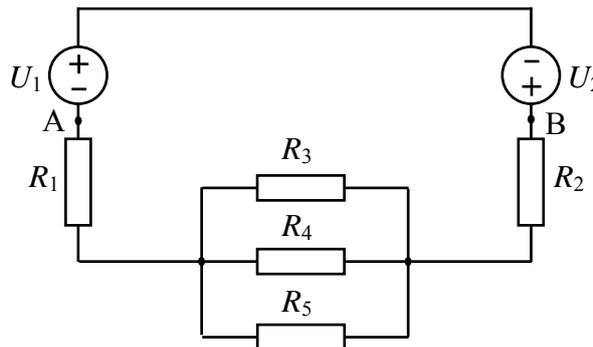
DATOS:  $U_1 = 20$  V,  $U_2 = 30$  V,  $R_1 = 2$   $\Omega$ ,  $R_2 = 1$   $\Omega$ ,  $R_3 = 10$   $\Omega$ ,  $R_4 = 20$   $\Omega$ ,  $R_5 = 30$   $\Omega$ .
