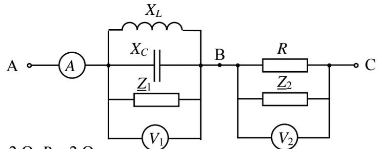
DATOS:  $\underline{Z}_1 = 3 - j4$   $\Omega$ ,  $\underline{Z}_2 = 1 + j3$   $\Omega$ ,  $X_L = 10$   $\Omega$ ,  $X_C = 2$   $\Omega$ ,  $R = 2$   $\Omega$
